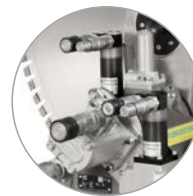
Robust saw head with standard hydraulic motors
